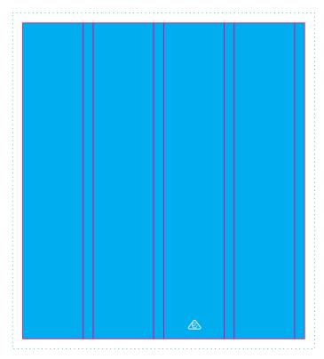
Blue shows max print area, 3mm bleed is required represented here by green dotted line. Pink line represents edges of the power bank and will not be printed. Grey shows button and will also not be printed
